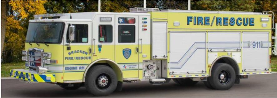
State of the art, best in class truck, provides either water or foam from a 1000-gallon tank, dispersing at 1500 gallons per minute. \$800k; 20+ yr life
