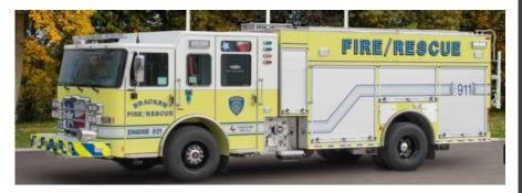
State of the art, best in class truck, provides either water or foam from a 1000-gallon tank, dispersing at 1500 gallons per minute. \$800k; 20+ yr life
